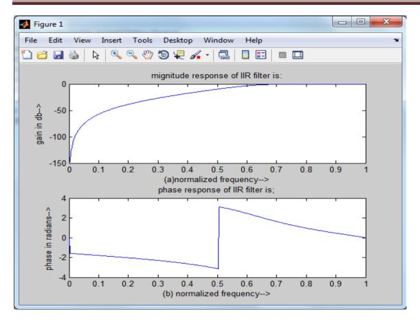
**RESULTS:** Hence magnitude and phase response of first order IIR Butter worth low pass and high pass filter was plotted in logarithmic scale by using a MATLAB Program successfully.
