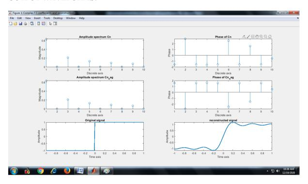
**RESULT**: Hence the Exponential Fourier series coefficients of a rectangular Periodic signal using MATLAB program was completed successfully.
