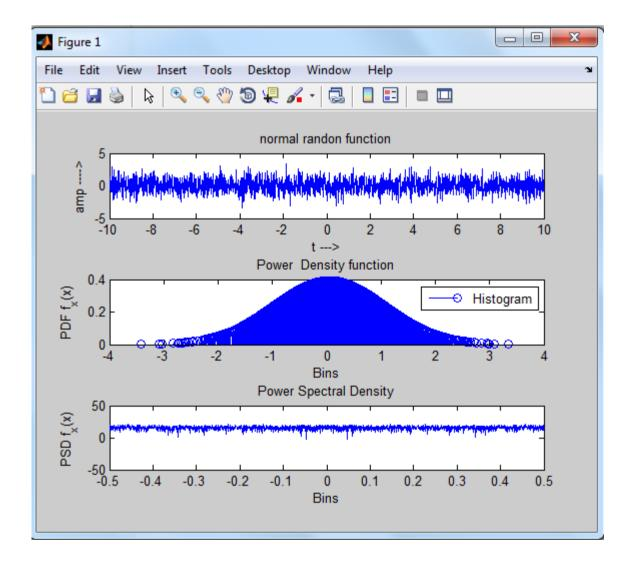
**RESULTS:** Hence Gaussian signal was generated and calculated the parameters such as Mean, Mean Square Value, Skew, Kurtosis, PSD and Probability Distribution Function by using MATLAB programming.
