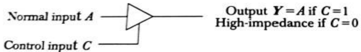
Figure 4-4 Graphic symbols for three-state buffer.
