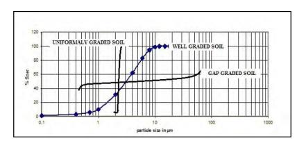
Gravels and sands may be either poorly graded (Uniformly graded) or well graded depending on the value of coefficient of curvature and uniformity coefficient.
