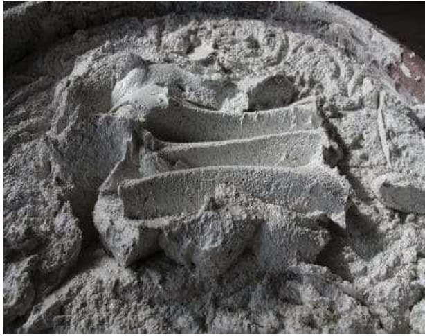
Fig 2: Mixing of cement and sand for plastering work.
