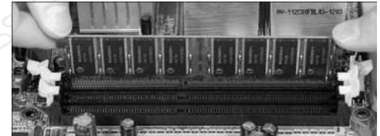
Inserting the RAM (Memory Chip) into the RAM Slots
