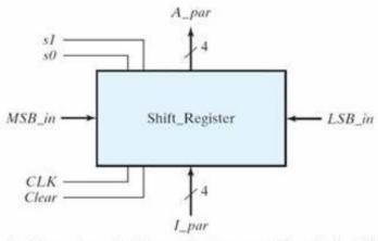
This is called the universal shift register because it has both shifts and parallel load capabilities.
