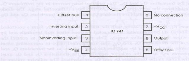
Fig. 1.59 8 Pin diagram
