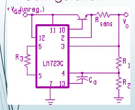
External pass transistor and current sensing added.
