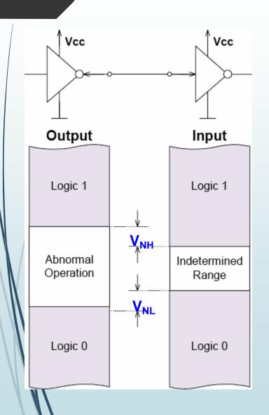
HI state noise margin:  $V_{NH} = V_{OH}(min) - V_{IH}(min)$
