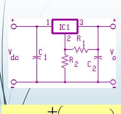
$$V_o = V_{reg} + \left( \frac{1}{R_1} + I_Q \right) R_2$$
