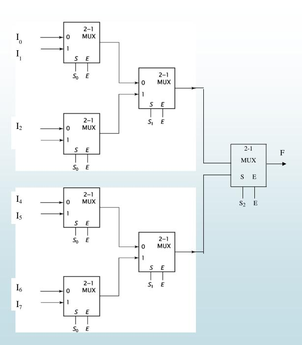
Example: Construct 8-to-1 multiplexer using one 2-to-1 multiplexer and two 4-to-1 multiplexers
