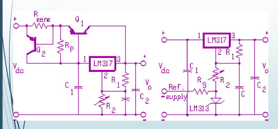
Circuit with pass transistor and current limiting
