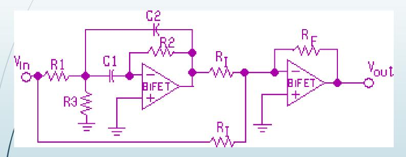
The equations for R1, R2, R3, C1, and C2 are the same as before.  $R = R_F$  for unity gain and is often chosen to be >> R1.
