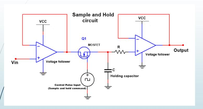
**Definition:** The Sample and Hold circuit is an electronic circuit which creates the samples of voltage given to it as input, and after that, it holds these samples for the definite time. The time during which sample and hold circuit generates the sample of the input signal is called sampling time.
