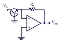
$$V_{out} \cong -R_f I_{EBO} anti \ln \left( \frac{V_{in}}{0.025} \right)$$
