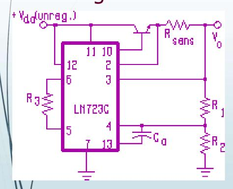
External pass transistor and current sensing added.
