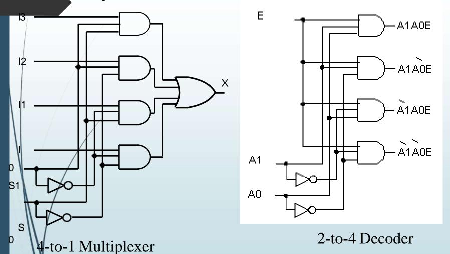
Note that the multiplexer has an extra OR gate.A1 andA0 are the two inputs in decoder. There are four inputs plus two selecs in multiplexer.
