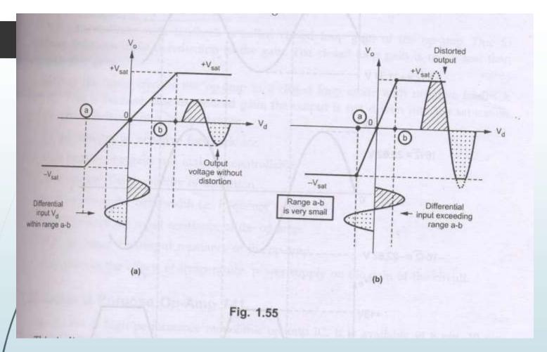
This indicates the inability of op-amp to work as a linear small signal amplifier in the open loop mode. Hence the op-amp in open loop configuration is not used for the linear applications
