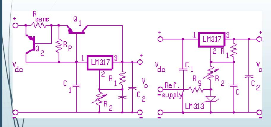
Circuit with pass transistor and current limiting
