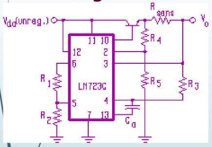
With external pass transistor and foldback current limiting
