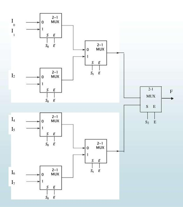
Example: Construct 8-to-1 multiplexer using one 2-to-1 multiplexer and two 4-to-1 multiplexers
