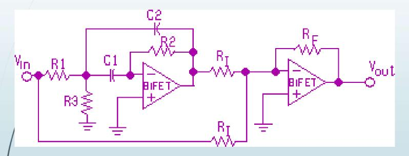
The equations for R1, R2, R3, C1, and C2 are the same as before.  $R_1 = R_F$  for unity gain and is often chosen to be >> R1.
