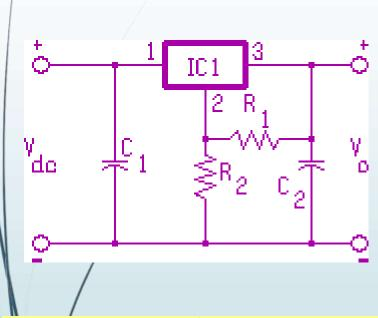
$$V_o = V_{reg} + V_{reg} + I_Q R_2$$
