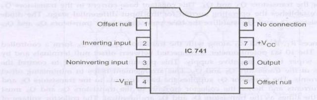
Fig. 1.59 8 Pin diagram
