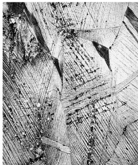
Initial recrystallization after 3 seconds @ 580°C
