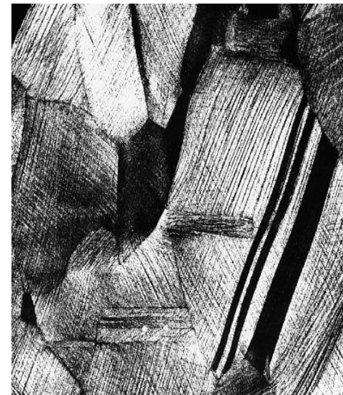
Cold Worked grains. Not annealed.
