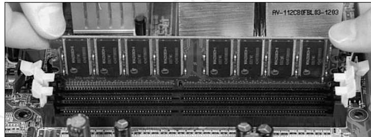
Inserting the RAM (Memory Chip) into the RAM Slots
