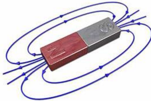
Fig: Field lines of a permanent magnet go from north to south.
