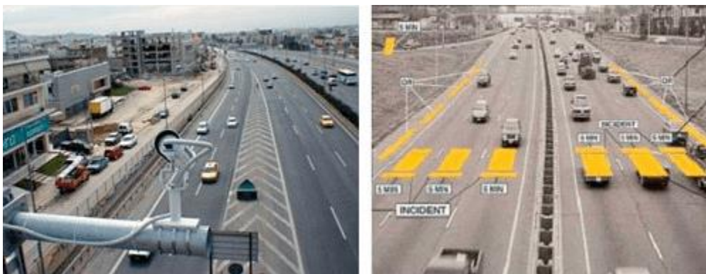
Left - normal traffic image | Right - a VIPS image with detection zones (source)
