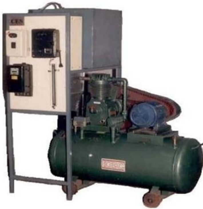
Pictorial view of multi stage air compressor
