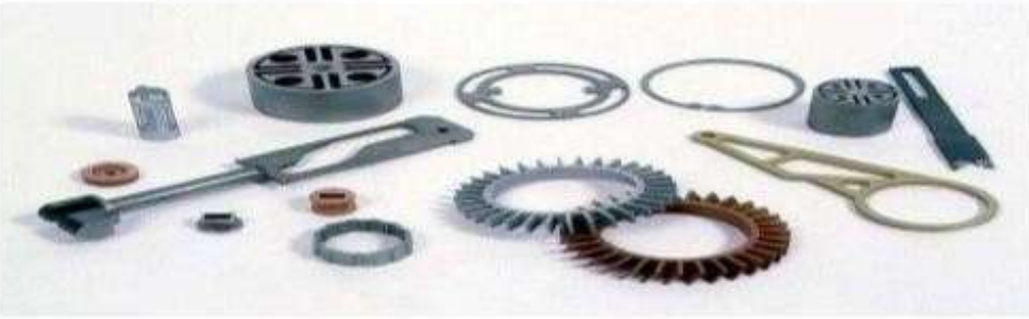
Figure: Difficult internal parts made by EDM process
